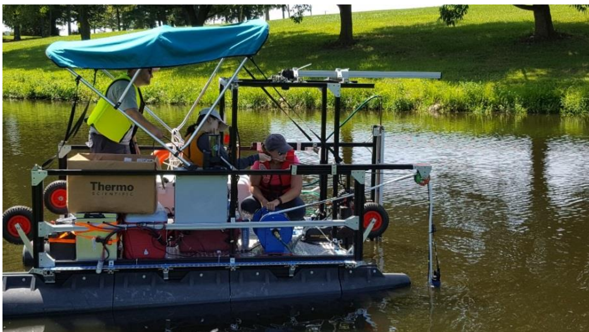
Figure: ARS designed, built and validated a GPS water sampling vehicle for irrigation water evaluation
